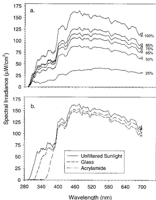
**FIGURE 1. Spectral irradiance for (a) unaltered sunlight and treatments with neutral density filtration designed to achieve relative intensities of 85%, 75%, 65%, 50%, and 25% sunlight; and (b) unaltered sunlight and treatments with glass and acrylamide filtration.**
